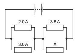
The current in three of the resistors is shown.
