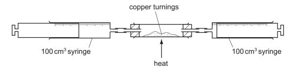
The gas was passed backwards and forwards over the heated copper turnings.
